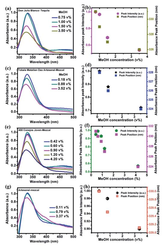
Fig. 7 UV-visible absorption spectra of NOCDs in the presence of some tested spiked branded and unbranded alcoholic beverages after dilution (a and b) Don Julio Blanco-Tequila (tDJB), (c and d) Tobala Matatlan Oax Artesanal (Traditional branded)-Mezcal (mTMOA), (e and f) 400 Conejos Joven-Mezcal (m400CJ) and (g and h) (traditional unbranded) Artesanal mezcal (mAR).
