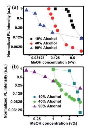
Fig. 4 Effect of NOCDs concentration on detection range: peak PL signal for different v% of MeOH at three different fixed v% of alcohols (EtOH + MeOH) measured at two different concentrations of NOCDs mimicking the real alcoholic beverages (such as Beer with 3-12%, Tequila: 40% and Vodka: 90%) (a) 8 μL NOCDs and (b) 70 μL NOCDs. (Normalized PL intensity vs. wavelength for each alcohol% is given in Fig. S5 and S6†).
