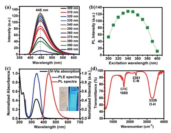
Fig. 1 (a) PL emission spectra of NOCD's at different excitation wavelengths, (b) variation of PL peak emission intensity at 445 nm as a function of different excitation wavelengths (maximas from (a) vs. excitation wavelength), (c) UV-vis absorption, PLE (corresponding to emission at 440 nm) and PL emission spectrum (excited at 340 nm); inset images are photographs of NOCDs in normal daylight and under 365 nm UV irradiation (d) FTIR spectrum corresponding to as prepared NOCDs.
