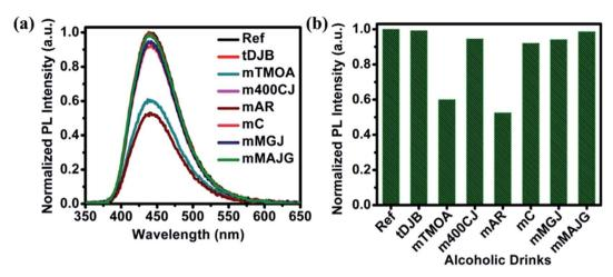
Fig. 5 Fluorescence response of NOCDs in the presence of diluted unspiked branded and unbranded alcoholic beverages (a) normalized PL emission measured at  $\lambda_{\rm ex} = 340$  nm (b) bar diagram representing the PL peak emission from NOCDs.
