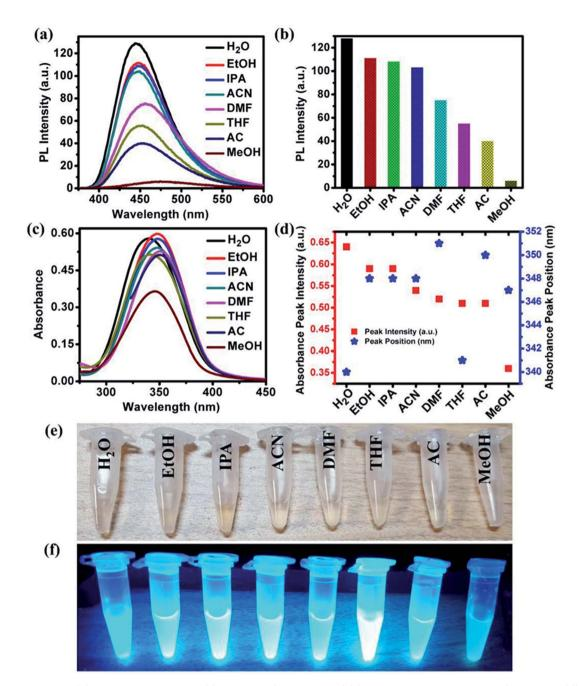
Fig. 2 Fluorescence of NOCDs in different solvents (a) PL spectra ( $\lambda_{\rm ex}=340$  nm) (b) variation in PL peak intensity (taken from (a)), (c) UV-vis absorption spectra, (d) peak absorption of NOCDs in different solvents, (e) photographs of NOCDs in different solvents under daylight and (f) NOCDs in different solvents irradiated by UV lamp ( $\lambda_{\rm ex}=365$  nm).
