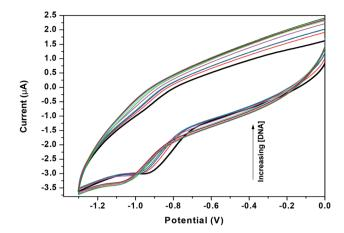
Fig. 4 Cyclic voltammograms for Zn(Onz) $_2$ Cl $_2$  in the absence (dark black line) and presence of different concentrations of calf-thymus DNA, [Zn(Onz) $_2$ Cl $_2$ ] = 100  $\mu$ M; [NaCl] = 120 mM; pH = 7.4; T = 301 K.
