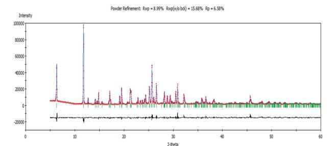
Fig. 1 The Rietveld refinement plot showing an agreement between the calculated and measured X-ray powder diffractograms of the complex.
