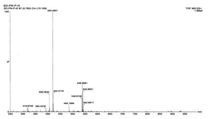
Fig. 3 Mass spectrum of the Zn(Onz)<sub>2</sub>Cl<sub>2</sub> complex
