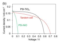
Fig. 4 (a) Schematic representation of the tandem cell power generation mechanism. (b) J-V curves under AM 1.5G (100 mW cm<sup>-2</sup>) of the tandem cell and individual n- and p-biophotovoltaic cells.
