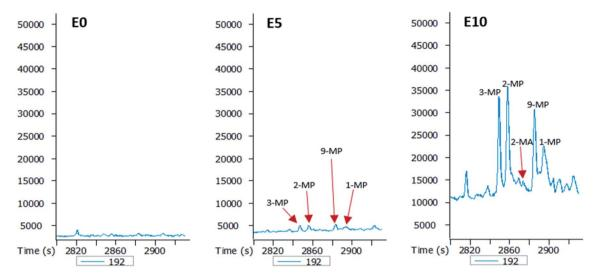
Fig. 6 Partial *m/z* 192 mass chromatograms of the E0, E5 and E10 leachates showing identification of methylphenanthrenes (MP) [E0: unblended diesel fuel; E5: diesel fuel containing 5% ethanol (v/v); E10: diesel fuel containing 10% ethanol (v/v)].
