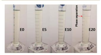
Fig. 1 Stability of four ethanol blends at 20 °C.
