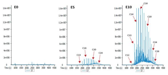
Fig. 4 Partial m/z 57 mass chromatograms of the E0, E5 and E10 leachates, showing identification of a homologous series of n-alkanes [E0: unblended diesel fuel; E5: diesel fuel containing 5% ethanol (v/v); E10: diesel fuel containing 10% ethanol (v/v); Cx: n-alkanes containing x number of carbon atoms].
