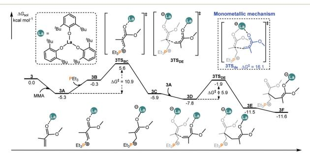
Fig. 4 Computed energy profiles for the 3/PEt<sub>3</sub> mediated (intermolecular RE/P systems) bimetallic pathway for MMA enchainment. Free energies (kcal mol<sup>-1</sup>) are relative to isolated reactants.
