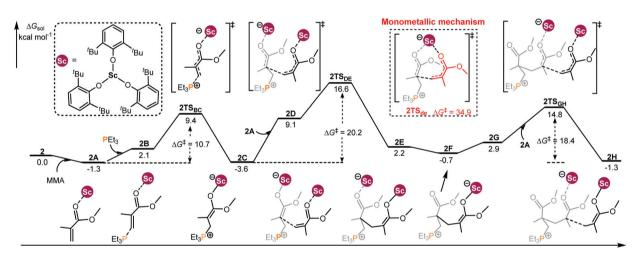
Fig. 2 Computed energy profiles for 2/PEt<sub>3</sub> mediated (intermolecular RE/P systems) bimetallic enchainment of MMA. Free energies (kcal mol<sup>-1</sup>) are relative to isolated reactants.
