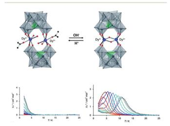
Fig. 7 (Up) Reversible SC-SC transformation between POM 1 and POM 2; (bottom) plots of  $\chi''(T)$  in the absence of a dc field for POM 1 (left) and POM 2 (right). Reproduced with permission from ref. 65. Copyright 2013 Royal Society of Chemistry. 65
