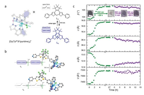
Fig. 1 (a) Molecular structure of  $[Dy(Tp^{py}) (pyridine)_2]PF_6$  in the cationic form and the open and closed form of the photoactive bispyridyl dithienylethene unit used in building 1c; (b) single crystal structures of 1c and 1o; (c) evolution of the unit cell parameters of 1c upon continuous irradiation with 532 nm light (green dots) followed by 365 nm light (purple dots). Reproduced with permission from ref. 49. Copyright 2020 American Chemical Society. 49
