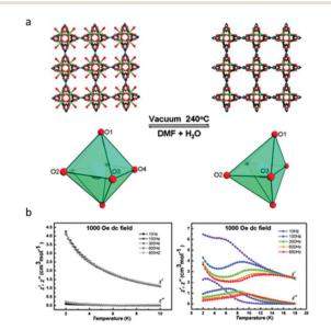
Fig. 4 (a) The structural or coordination geometry changes of the framework and Dy(III) ions; (b) temperature dependence of  $\chi'$  and  $\chi''$  for Dy(BTC)(H2O)·DMF (left) and Dy(BTC) (right). Reproduced with permission from ref. 61. Copyright 2013 Royal Society of Chemistry. 61
