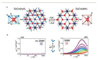
Fig. 5 (a) Crystal structures and (b) plots of  $\chi''(v)$  in the absence of a dc  $field \ for \ \{[Dy(III)(H_2O)_2][Co(III)(CN)_6]\} \cdot 2.2H_2O \ (left) \ and \ \{Dy(III)[Co(III)(CN)_6]\} \cdot 2.2H_2O \ (left) \ and \ (le$ (right). Reproduced with permission from ref. 63. Copyright 2019 American Chemical Society. 63
