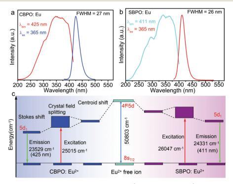
Fig. 3 Room temperature excitation and emission spectra of (a) Ca<sub>2</sub>Be<sub>2</sub>(PO<sub>4</sub>)<sub>2</sub>:Eu<sup>2+</sup> and (b) Sr<sub>2</sub>Be<sub>2</sub>(PO<sub>4</sub>)<sub>2</sub>:Eu<sup>2+</sup> phosphors. (c) Schematic energy level diagram for  $Eu^{2+}$  ion in  $Ca_2Be_2(PO_4)_2$  and  $Sr_2Be_2(PO_4)_2$  crystal structures.
