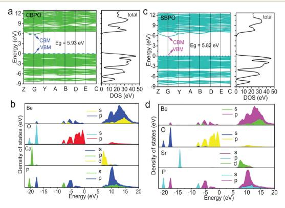
Fig. 2 The calculated energy band structure as well as the total density of states of (a) Ca<sub>2</sub>Be<sub>2</sub>(PO<sub>4</sub>)<sub>2</sub> and (c) Sr<sub>2</sub>Be<sub>2</sub>(PO<sub>4</sub>)<sub>2</sub> host. The partial (Be, Ca, P, and O atoms) density of states for (b) Ca<sub>2</sub>Be<sub>2</sub>(PO<sub>4</sub>)<sub>2</sub> and (d) Sr<sub>2</sub>Be<sub>2</sub>(PO<sub>4</sub>)<sub>2</sub>.
