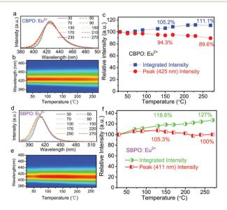
Fig. 4 Temperature-dependent emission spectra of (a and b)  $Ca_2Be_2(PO_4)_2$ :  $Eu^{2+}$  and (d and e)  $Sr_2Be_2(PO_4)_2$ :  $Eu^{2+}$  phosphors in the temperature range of 30-270 °C. Temperature-dependent normalized integrated emission spectra and maximum emission peak intensity of (c)  $Ca_2Be_2(PO_4)_2$ :  $Eu^{2+}$  and (f)  $Sr_2Be_2(PO_4)_2$ :  $Eu^{2+}$  phosphors.
