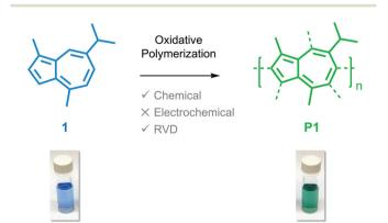
Scheme 1 The oxidative polymerization of quaiazulene (1) to poly (guaiazulene) (P1).
