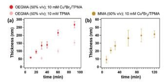
Fig. 1 Dry thickness of polymer brushes synthesized by SI-Zn<sup>0</sup>-ATRP and measured by VASE. (a) Dry thickness of POEGMA brushes after different polymerization times, using a 50% OEGMA (v/v) solution in DMF, 10 mM TPMA, with and without 10 mM Cu<sup>II</sup>Br<sub>2</sub>. (b) Dry thickness of PMMA brushes synthesized by using a mixture of 50% MMA (v/v) in DMF, and 10 mM Cu<sup>II</sup>Br<sub>2</sub>/TPMA. Values of dry thickness are expressed as mean  $\pm$  SD (n = 4).
