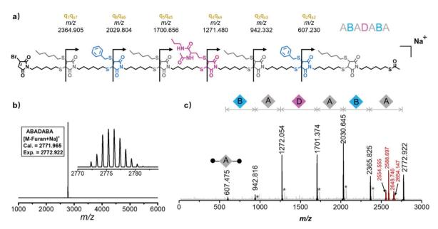
Fig. 5 (a) Illustration of the theoretical fragmentations of ABADABA. (b) The MALDI-TOF MS spectrum and (c) MALDI-TOF MS/MS spectrum of ABADABA. \*Signals arise from concomitant fragmentations, detailed in the ESI (Table S7†).
