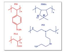
Fig. 13 Ionic polymers used by Yuan et al. to design tough hydrogels. Adapted with permission from ref. 113. Copyright 2019, American Chemical Society.
