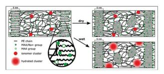
**Fig. 9** Schematic morphological solid-state evolution of sodium neutralized poly(ethylene-*ran*-methacrylic acid) (E/MAA-Na<sup>+</sup>) ionomers under thermal annealing. Reprinted with permission from ref. 86. Copyright 1995, American Chemical Society.
