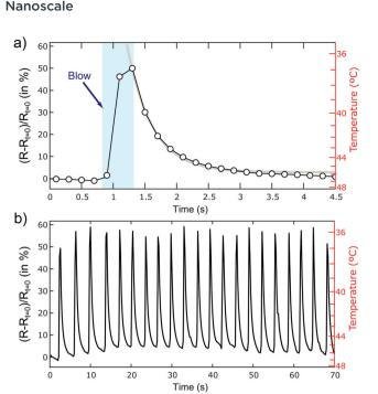
Fig. 5 Response time of WS<sub>2</sub>-on-paper thermoresistive devices upon sudden temperature changes. (a) Resistance change vs. time of a WS<sub>2</sub>-on-paper device subjected to a sudden change in temperature. The device is warmed up to ~45 °C and at time t ~ 1 s a hand pump blows cool air onto the device. (b) 21 blowing cycles to demonstrate the reproducibility of the thermoresistive device.
