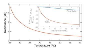
Fig. 4 Temperature dependence of the resistance of WS2-on-paper thermoresistive devices. (a) Resistance vs. temperature for a WS2-onpaper device with pencil-drawn interdigitated devices. (inset) Comparison between the resistance vs. temperature curves measured for the WS<sub>2</sub> and a graphite thermoresistive devices on paper.
