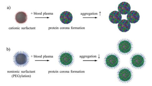
Fig. 6 Schematic illustration of the aggregation state of SiO<sub>2</sub> NCs stabilized with cationic surfactant CTMA-Cl and nonionic surfactant Lutensol AT50.
