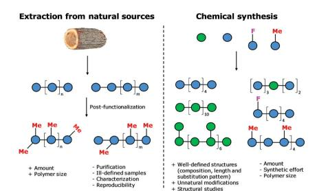
Fig. 2 Comparison of extraction and chemical synthesis used to produce polysaccharide materials.
