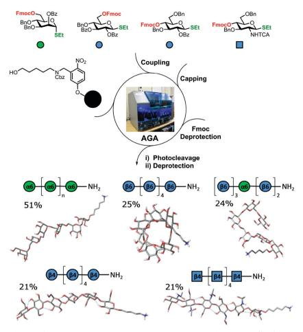
Fig. 3 AGA of a collection of well-defined oligosaccharides revealing that some polymers form helices (β-1,6 glucosides), some adopt rod-like structures ( $\beta$ -1,4 oligomers), while others lack a defined conformational structure ( $\alpha$ -1,6 mannosides). Isolated yields after AGA, deprotection, and purifications are shown.
