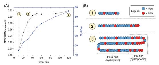
Fig. 4 (A) Evolution of the PPG: HMDI molar ratios and GPC molecular weight of ZDTC-catalysed PU as a function of time; (B) illustration of PEG-PPG distribution in the ZDTC-catalysed polymer at different timepoints during the reaction.
