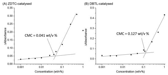
Difference in DPH absorbance at 376 and 394 nm as a function of polymer concentration for PUs catalysed by (A) ZDTC and (B) DBTL. The CMC of the polymer was determined by the intersection of the extrapolated linear best fit lines at low and high concentrations of polymer.
