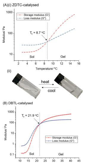
**Fig. 2** Oscillatory temperature sweep showing the changes in storage (G') and loss modulus (G'') as a function of temperature, as well as the gelation temperature of 10 wt% PU catalysed by (A) ZDTC and (B) DBTL. Figure (A)(ii) shows the reversible sol–gel transition of a transparent 10 wt/v% solution of ZDTC-catalysed PU in water.
