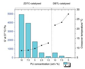
Fig. 3 Chart showing the storage moduli (G', left vertical axis, bars) and crossover temperatures ( $T_{\rm c}$ , right vertical axis, filled dots) of different concentrations of PU, whose syntheses are catalysed by either ZDTC or DBTL. At concentrations of <5.0 wt/v%, the DBTL-catalysed PUs do not form gels below 40 °C.
