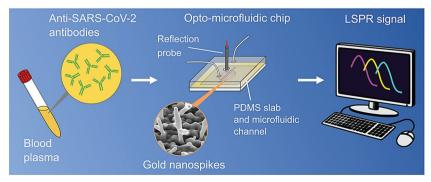
Fig. 6 An opto-microfluidic sensing platform prepared for the rapid detection of antibodies against the SARS-CoV-2 spike protein in diluted human plasma with remarkable sensitivity. The sensing principle is based on LSPR, involving gold nanospikes in a microfluidic device, coupled with an optical probe. Reproduced with permission from ref. 51.
