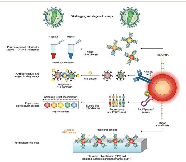
Fig. 3 Nano-based sensors for the detection of SARS-CoV-2 based on viral tagging and diagnostic assays: Ab, antibody; FRET, Förster resonance energy transfer; LSPR, localized surface plasmon resonance; NPs, nanoparticles; PNA, peptide nucleic acid; and PPT, photothermal therapy. Reproduced with permission from ref. 21.
