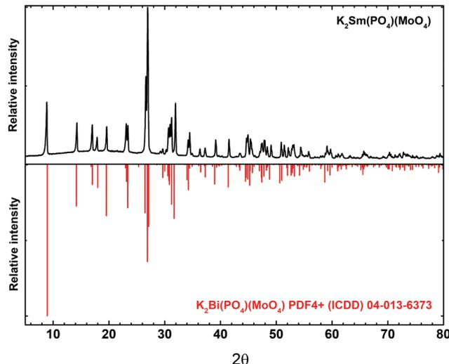
Fig. 1 XRD patterns of  $\text{K}_2\text{Sm}(\text{PO}_4)(\text{MoO}_4)$  and  $\text{K}_2\text{Bi}(\text{PO}_4)(\text{MoO}_4)$  reference.
