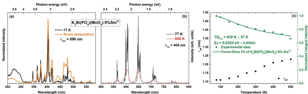
Fig. 5 Temperature dependent excitation ( $\lambda_{em} = 598$  nm) and (b) emission ( $\lambda_{ex} = 404$  nm) spectra of  $K_2Bi(PO_4)(MoO_4):Sm^{3+}$ , (c) calculation of  $TQ_{1/2}$  value for the sample doped with 5%  $Sm^{3+}$  from normalized emission intensity and  $\tau_{eff}$  values calculated from temperature dependent decay curves.
