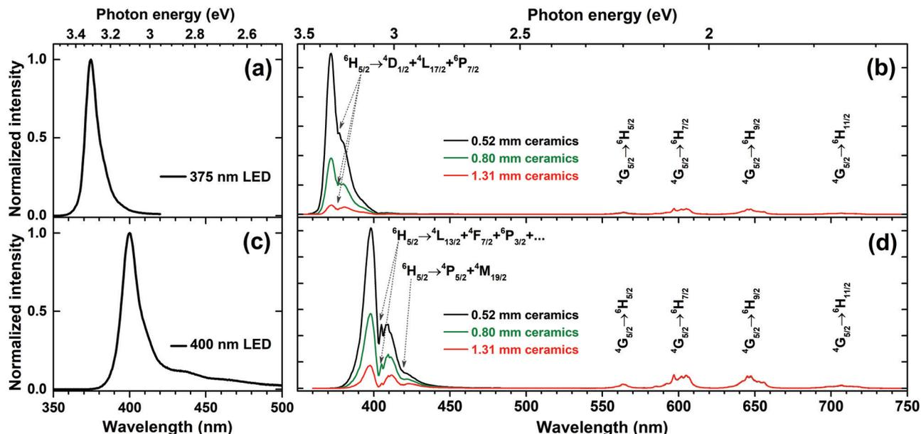
Fig. 8 Emission spectra of (a) 375 nm LED, (c) 400 nm LED. Emission spectra of  $\text{K}_2\text{Bi}(\text{PO}_4)(\text{MoO}_4):5\%\text{Sm}^{3+}$  ceramic discs excited with (b) 375 nm LED, and (d) 400 nm LED.
