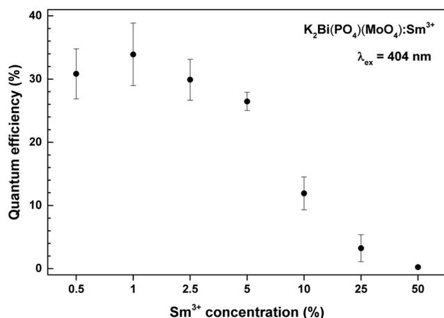
Fig. 7 Quantum efficiencies of K<sub>2</sub>Bi(PO<sub>4</sub>)(MoO<sub>4</sub>):Sm<sup>3+</sup> phosphors as a function of Sm<sup>3+</sup> concentration.
