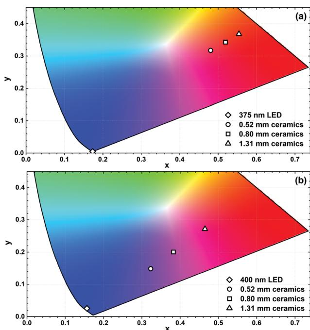
Fig. 9 Fragments of the CIE 1931 colour space diagram with colour coordinates of  $\text{K}_2\text{Bi}(\text{PO}_4)(\text{MoO}_4):5\%\text{Sm}^{3+}$  ceramic disks combined with 375 nm (a) and 400 nm (b) emitting LEDs.
