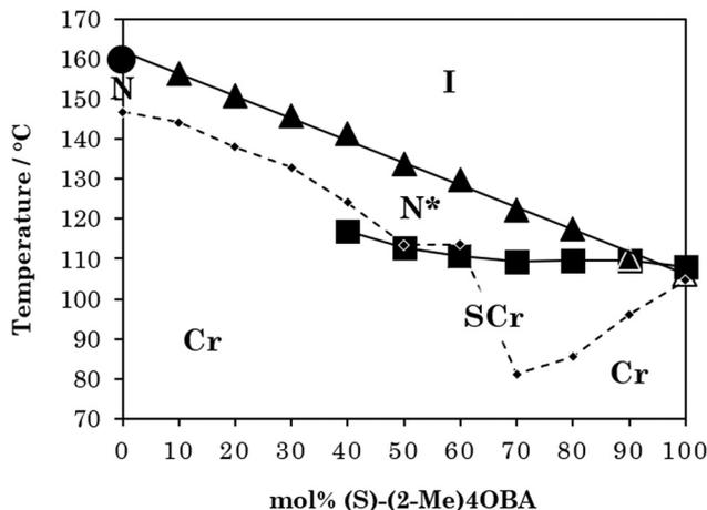
Fig. 2 Phase diagram of binary mixtures of 4OBA and (S)-(2-Me)4OBA, where  $\blacklozenge$  represents the melting point,  $\bullet$   $T_{NI}$ ,  $\blacktriangle$   $T_{N^*}$ , and  $\blacksquare$   $T_{SCrNI}$ . An unfilled triangle represents a virtual transition temperature.
