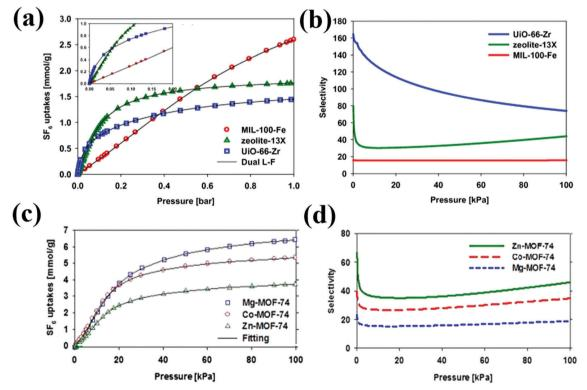
Fig. 1 SF<sub>6</sub> pure gas adsorption isotherms and selectivity calculated using IAST theory on (a) & (b) MIL-100-Fe, 13X zeolite, and UiO-66(Zr); (c) & (d) M-MOF-74 (M = Mg, Co, Zn) at 298 K, respectively.<sup>25,32</sup> Reproduced from ref. 25 and 32 with permission from Elsevier.
