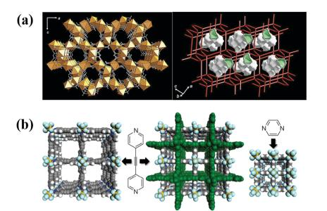
Fig. 7 (a) X-ray crystal structure and crystal topology of Mn(COO)<sub>2</sub>.55 (b) Structures of SIFSIX-Cu, interpenetrated SIFSIX-Cu-i and pore contracted SIFSIX-3-Zn. 55,57 Reproduced from ref. 55 and 57 with permission from The Royal Society of Chemistry & Springer Nature.
