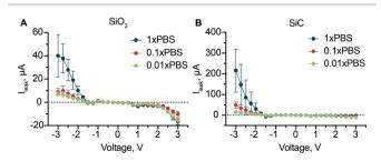
Fig. 4 Gate leakage current. Gate leakage current at different solution concentrations for SiO<sub>2</sub> dielectric layer (A) and SiC dielectric layer (B).
