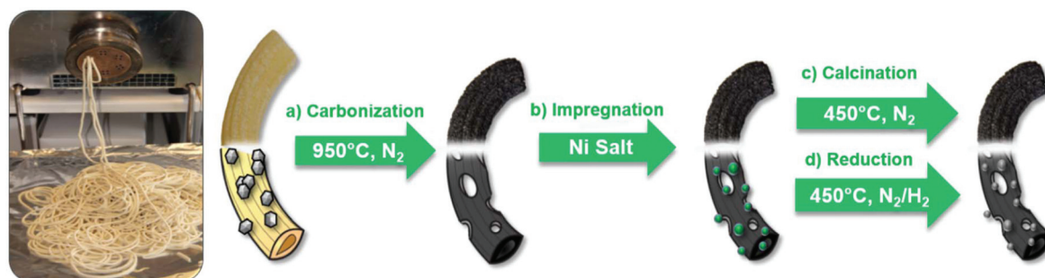
Fig. 3 Schematic representation of the catalyst synthesis protocol starting from the extrusion, carbonization, calcination, and reduction steps.
