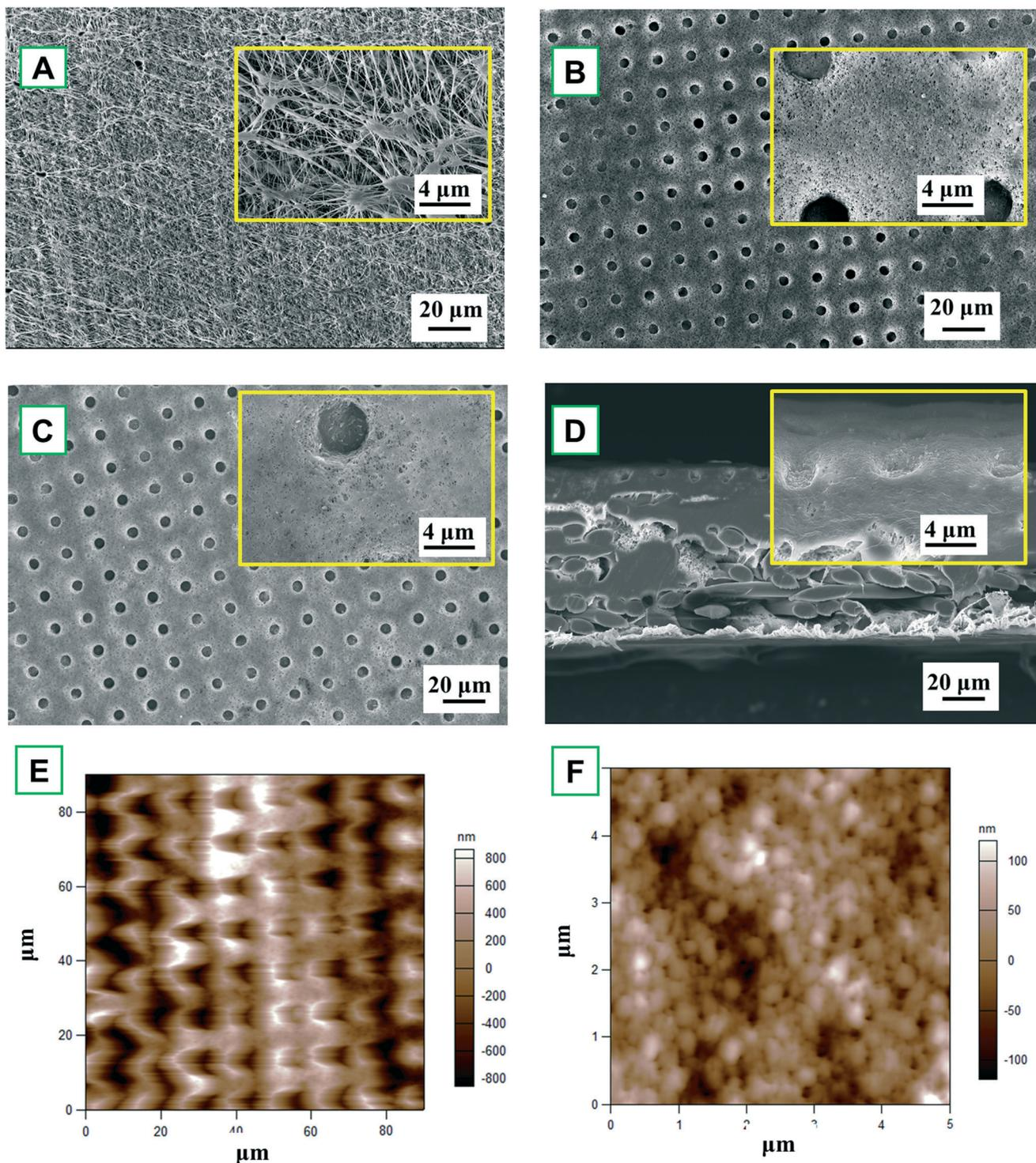
**Fig. 2** SEM images of the membrane surface: (A) pristine PTFE (C-PTFE); (B)  $\text{TiO}_2$  atomic layer deposited nanoimprinted membrane (ALD); (C) fluorinated ALD membrane (FTES); (D) cross-section of FTES. Atomic force microscopy (AFM) images of (E) the membrane surface demonstrating the dot pattern and (F) deposition layer of  $\text{TiO}_2$ .
