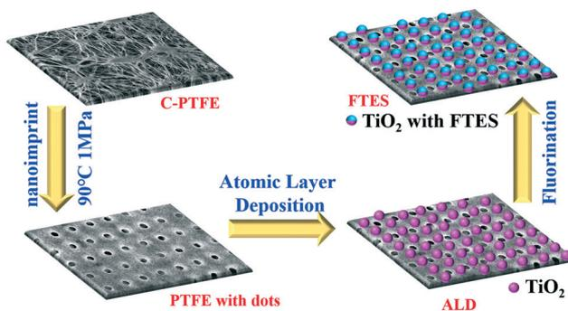
Fig. 1 Schematic illustration of design and procedures for fabricating the nanoimprint PTFE membrane with a fluorinated TiO<sub>2</sub> deposition layer.
