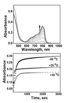
Fig. 4 Top: Spectral changes associated with the catalytic reduction of dioxygen by Co<sub>4</sub>L1 (0.04 mM) in the presence of Fc\* and TFA. Bottom: Time profiles of the formation of Fc\*+ monitored at 780 nm during the reduction of O2 (0.18 mM) by Fc\* (3 mM) and Co4L1 (0.04 mM) in the presence of TFA (10 mM) in acetone at 30 °C, 25 °C as well as at -50 °C.
