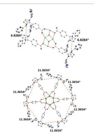
Fig. 1 Comparison of the distances between the metal binding sites in L1 (top) and L2 (bottom). X-ray crystal structure of L1 and L2 with 30% ellipsoid probability of the atoms. Hydrogen atoms and the n-butyl ("Bu-) groups on the tin atoms have been omitted for clarity. Color code: nitrogen-blue; carbon-grey; oxygen-red; tin-green.
