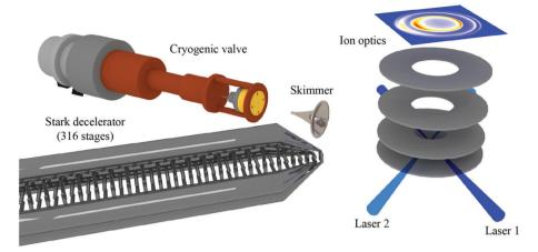
Fig. 1 Schematic representation of a crossed beam apparatus. A beam of NO radicals is passed through a Stark decelerator and scattered with a pulsed beam of para-H2 or ortho-D2. The inelastically scattered NO radicals are state-selectively ionised using two pulsed lasers and detected using velocity map imaging. Only the last section of the Stark decelerator is shown. Reprinted with permission from Gao et al.,58 copyright 2017 American Chemical Society.
