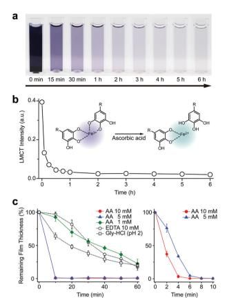
Fig. 1 (a) Time-lapse optical images of the  $Fe^{3+}$ -TA MPC solution after addition of ascorbic acid at 0 min (10 mM). (b) Graph of LMCT intensity at 565 nm versus reaction time. (c) Graphs of film thickness versus reaction time. The Fe<sup>3+</sup>-TA MPC film was incubated in an aqueous solution of AA (1, 5, or 10 mM), EDTA (10 mM), or gly-HCl buffer (pH 2). The right graph for AA (5 and 10 mM) is the enlarged one for the first 10 min of incubation.
