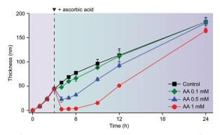
Fig. 4 Graphs of film thickness versus reaction time in the IGI-based solution ( $[Fe^{2+}] = 10 \text{ mM}$ , [TA] = 1 mM). AA (0.1, 0.5, or 1 mM) was added to the solution after 3 h of reaction.
