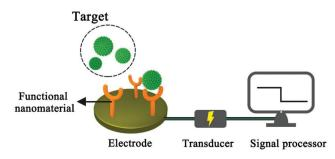
Fig. 1 Schematic diagram of an electrochemical sensor
