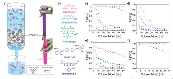
Fig. 2 (a) Schematic representation and digital photograph of column separation using  $\beta$ -CD-PN as the adsorbent (flow rate  $\sim 0.4$  mL s<sup>-1</sup>); (b) structures of tested small molecular dyes; column dye adsorption data of (c)  $\beta$ -CD-PN (d)  $\alpha$ -CD-PN (e) Glu-PN and (f) activated carbon (C = eluent concentration,  $C_0$  = feed concentration). In Fig. 2f, all dye adsorption data are overlapping except for Congo red.
