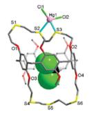
Fig. 2 The exo-coordinated mercury(II) chloride complex [HgCl<sub>2</sub>(CH<sub>2</sub>Cl<sub>2</sub>@ $\mathbf{L}$ )] (1).
