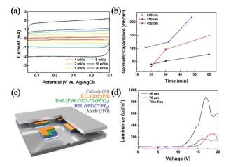
Fig. 3 (a) Cyclic voltammograms of 450 nm PEDOT:PF $_6$  (146 NPs) decorated carbon UME at different scan rates. (b) Geometric capacitance (mF cm $^{-2}$ ) of PEDOT NPs decorated electrodes (200 nm-black, 350 nm-red, and 450 nm-blue). (c) Schematic representation of an OLED device investigated in this work. (d) Luminescence measurements from OLED devices employing PEDOT:PF $_6$  NPs (40 and 70 nm) and a PEDOT:PF $_6$  thin film (deposited by cyclic voltammetry) as hole transport layers.
