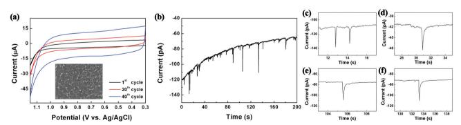
Fig. 1 (a) Electropolymerization of EDOT by cyclic voltammetry (0.1 M EDOT, 0.2 M TBAP in DCM at 50 mV s<sup>-1</sup> scan rate; inset displays resultant film by SEM). (b) Chronoamperogram exhibiting collision signals of 200 nm droplets onto a 10 µm carbon electrode, with each oxidation spike leading to a synthesized PEDOT NP. (c)-(f) Typical single droplet electrolysis signals. See also Fig. S2 and S3 (ESI†).
