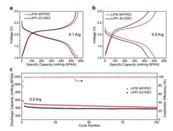
Fig. 2 Li||SPAN half-cell performance in different electrolytes at room temperature. Voltage curves at (a)  $0.1\,\mathrm{A}~\mathrm{g}^{-1}$  and (b)  $0.5\,\mathrm{A}~\mathrm{g}^{-1}$ ; (c) long-term cycling performance at  $0.5\,\mathrm{A}~\mathrm{g}^{-1}$ .
