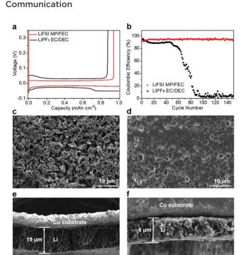
Fig. 1 Li metal performance in the selected electrolytes at room temperature. (a) Li plating/stripping curves and (b) long-term cycling performance of Li||Cu cells in LiFSI MP/FEC, and LiPF $_6$  EC/DEC at 0.5 mA cm $^{-2}$ ; top (c and d) and cross-section (e and f) views of the SEM images of Li deposits obtained in LiPF $_6$  EC/DEC (c and e) and LiFSI MP/FEC (d and f) at 1 mA h cm $^{-2}$  and 0.5 mA cm $^{-2}$ .
