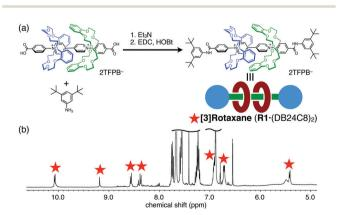
Fig. 4 (a) Reaction scheme of [3]rotaxane R1:(DB24C8)<sub>2</sub> formation by amide formation, and (b) <sup>1</sup>H NMR spectrum of the reaction mixture (400 MHz, CDCl<sub>3</sub>/CD<sub>3</sub>CN (4:1)).
