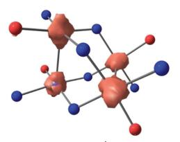
Fig. 2 Unpaired spin density plot for  $[Ni_4]^{4+}$ . The isocontour value is set to the default (0.03).
