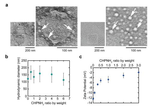
Fig. 3 The characterization of CHPNH<sub>2</sub> nanogel/exosome hybrids. (a) TEM images of the nanogel/exosome hybrid (left) and nanogel (right). Some of the nanogels are indicated by white arrows. (b) Distribution of the hydrodynamic diameter of hybrids at various weight ratios of the nanogels by NTA. (c)  $\zeta$ -Potential of hybrids (exosome with a protein concentration of 3  $\mu$ g mL<sup>-1</sup>) at various weight ratios of nanogels.
