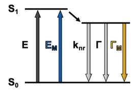
Fig. 1 Jablonski diagram for (a) a fluorophore excited in free-space conditions and (b) modified pathways in the vicinity of a plasmonic nanoparticle. E: excitation,  $k_{nr}$ : cumulative non-radiative decay rate,  $\Gamma$ : radiative decay rate. The M subscript represents metal-enhanced routes.
