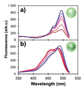
Fig. 6 Excitation spectra of (a) 80 nm  $SiO_2$  NPs and (b) Ag@SiO<sub>2</sub> NPs (60 nm core and 12 nm shell) functionalized with FL derivatives ( $\lambda_{em}$  = 540 nm). pH values of the phosphate buffers range incrementally from 5.9 (red) to 7.6 (blue).
