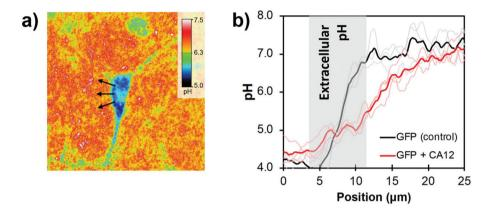
Fig. 12 (a) 2D pH cartography of a GFP (green fluorescent protein) + CA12 transfected cardiac fibroblast on the pH-responsive surface with  $\lambda_{\rm exc}$  = 489  $\pm$  6 nm/436  $\pm$  5 nm and  $\lambda_{\rm em}$  = 536  $\pm$  20 nm. (b) pH measured as a function of the distance from the cell center (arrows in c) for an unaltered cell (control with GFP) and the GFP + CA12 transfected fibroblast. Adapted from ref. 115 with permission from the Royal Society of Chemistry, Copyright 2014.
