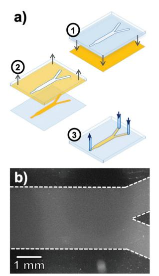
Fig. 13 (a) Fabrication steps for the pH-sensitive microfluidic Y-channel including (1) contact of the plasma-activated PDMS stamp with the Age (FL) coated glass coverslip, (2) removal of the nanoparticle-bound stamp and (3) deposition of the PDMS microfluidic channel on the patterned glass surface. (b) Fluorescence image of the pH-sensitive channel after the stamping process. Adapted from ref. 123 with permission from the Royal Society of Chemistry, Copyright 2016.
