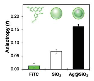
Fig. 5 Fluorescence anisotropy values measured at 20 °C for molecular fluorescein isothiocyanate (FiTC), encapsulated SiO<sub>2</sub> NPs (80 nm), and 80 nm Ag core-15 nm silica shell MEF architectures functionalized with a FL derivative ( $\lambda_{\rm exc}$  = 485 nm,  $\lambda_{\rm em}$  = 520 nm).
