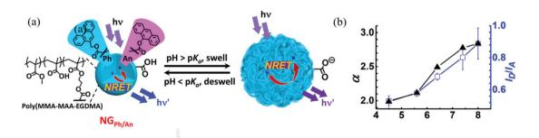
Fig. 3 (a) Schematic depicting the sensing mechanism of pH-responsive nanogel probes (NGPh/An). (b) Variation of the average linear swelling ratio ( $\alpha$ ) and  $I_D/I_A$  with pH for DX NG(NGPh/An). Reprinted (adapted) with permission from ref. 67. Copyright (2017) American Chemical Society.
