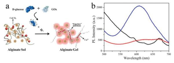
Fig. 6 (a) Schematic illustration of the glucose sensor using hybrid CuNC-alginate; (b) PL spectra of Cu NCs (red), Cu NCs + alginate (black), and CuNCs + alginate + glucose + GOx (blue). Reprinted (adapted) with permission from ref. 97. Copyright (2019) American Chemical Society.
