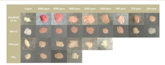
Fig. 2 The visual color changes of SiO<sub>2</sub>@MCM-41, SBA-15, silica gel and SiO<sub>2</sub> in response to different concentrations of SO<sub>2</sub> gas.
