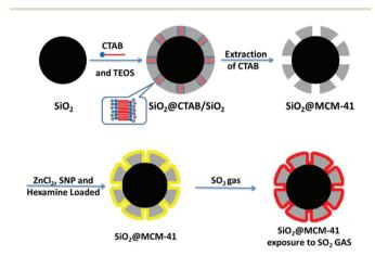
Scheme 1 Schematic illustration of the fabrication and detection processes of SiO2@MCM-41.
