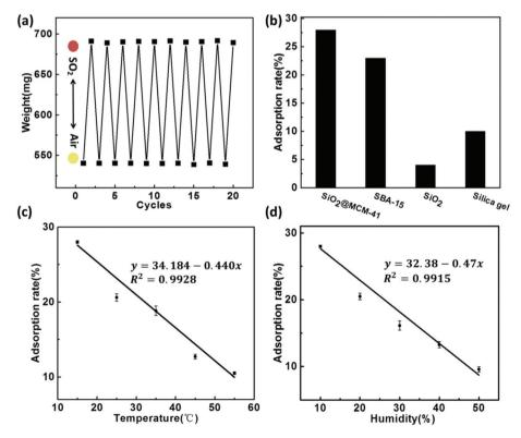
Fig. 3 (a) Reversible changes of the weight of SiO<sub>2</sub>@MCM-41 when alternately exposed to air and SO<sub>2</sub> gas, and the corresponding color changes. (b) The adsorption rates of SiO<sub>2</sub>@MCM-41, SBA-15, silica gel and SiO<sub>2</sub> toward SO<sub>2</sub> gas. (c) The relationship between the adsorption rate and the temperature of  $SO_2$  gas. (d) The relationship between the adsorption rate and the humidity of  $SO_2$  gas.
