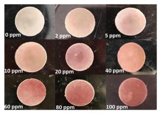
Fig. 4 The visual color changes of SiO<sub>2</sub>@MCM-41 discs in response to low concentrations of SO<sub>2</sub> gases.
