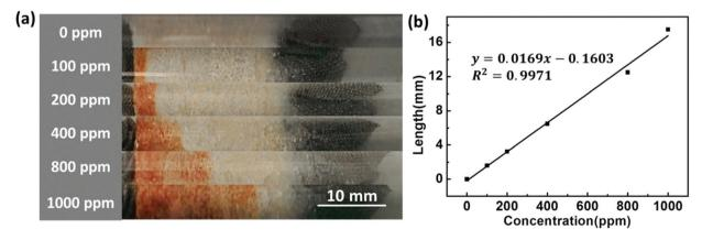
Fig. 5 (a) The visual color change length and (b) corresponding fitting curve of the SO<sub>2</sub> GDT in response to various concentrations of SO<sub>2</sub> gases.
