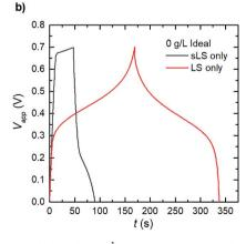
Fig. 5 Simulated electrode response under galvanostatic charge—discharge at  $1689 \,\mu\text{A}$  (2 A g<sup>-1</sup>) for 1\_2 electrodes. (a) At steady operation (after long cycling), and (b) for idealized cases where LS is confined in electrode domain in only solid (sLS) or dissolved (LS) form.
