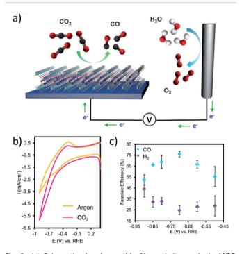
Fig. 9 (a) Schematic showing a thin film cobalt–porphyrin MOF,  $Al_2(OH)_2TCPP$ -Co, performing  $CO_2$  reduction. (b) An increase in current is observed in the cyclic voltammogram when the MOF is subjected to a  $CO_2$  environment. (c) Selectivity for generation of CO and  $H_2$  was tested over the potential range -0.5 to -0.9 V vs. RHE with a reported peak faradaic efficiency for CO of 76%. Adapted with permission. <sup>158</sup> Copyright 2015 American Chemical Society.
