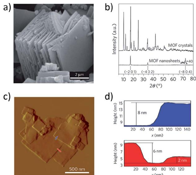
**Fig. 8** (a) SEM image of bulk CuBDC MOF crystals comprised of layered nanosheets. (b) pXRD scans of bulk CuBDC MOF crystals and corresponding nanosheets. (c) AFM map of MOF nanosheets. (d) Height profiles taken along the paths indicated in (c). Adapted by permission from Springer Nature.<sup>75</sup> Copyright 2015.
