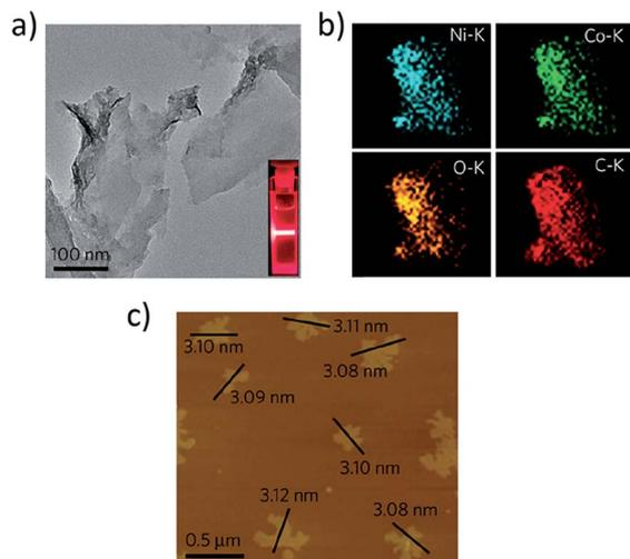
**Fig. 7** (a) TEM image of NiCo-UMOFNs with optical image of Tyndall light scattering (inset) upon laser irradiation. (b) EDS elemental mapping of NiCo-UMOFNs obtained within a TEM. (c) AFM map of individual NiCo-UMOFN flakes. Adapted by permission from Springer Nature.<sup>115</sup> Copyright 2016.
