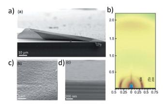
Fig. 5 (a) Highly uniform thin film of LZU-1 synthesized with *in situ* deprotection. (b) The crystallinity and orientation are confirmed by GIWAXS. (c) The thin film is composed of small crystallites with similar orientation and is 190 nm thick as measured by (d) cross-sectional SEM. Adapted with permission.<sup>101</sup> Copyright 2017 American Chemical Society.
