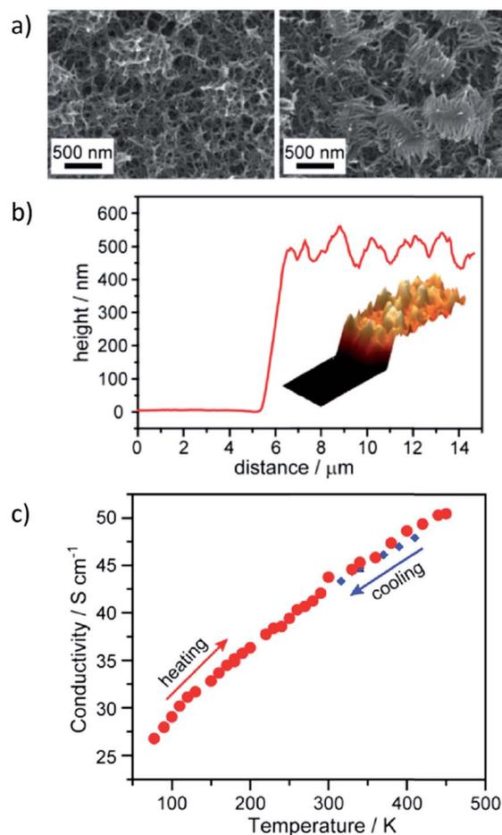
Fig. 10 a) SEM micrographs of  $\text{Ni}_3(\text{HITP})_2$  films with 500 nm thickness measured *via* (b) AFM. (c) van der Pauw conductivity measurements at various temperatures show reversible increase in conductivity for 500 nm thick films on quartz. Adapted with permission.<sup>168</sup> Copyright 2014 American Chemical Society.
