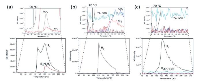
Fig. 3 Evolved gas mass spectra vs. temperature (RT – 250 °C) of: (a) as-received AB; (b) 1:1 AB: GO composite and (c) 1:2 AB: rGO composite. <sup>38</sup>Ar is present at approximately constant partial pressure in the TG-DTA-MS gas stream in all experiments.
