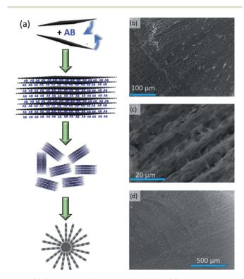
Fig. 1 (a) Schematic of the assembly of AB-GO composite beads where sandwich-like GO/AB layers rearrange radially during icetemplating; SEM images of the radial structure of: (b), (c) GO and (d) AB-GO composite.
