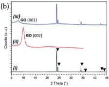
Fig. 2 (a) STEM image of 1:2 AB: rGO composite showing a larger cluster of AB among rGO sheets; (b) PXD patterns of: (i) as-received AB, (ii) ice-templated GO beads; (iii) 5:4 AB: GO nanocomposite. AB reflections are indicated by triangles.
