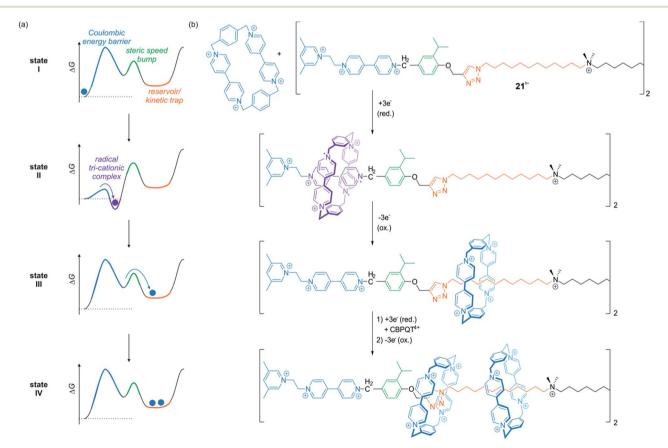
Fig. 18 Operation sequence of Stoddart's electrochemically driven molecular pump: (a) simplified energy landscapes of translational wheel motion along axle  $21^{8+}$  in states I–IV. (b) Structure of the axle  $21^{8+}$ , the CBPQT<sup>4+</sup> wheel and corresponding (pseudo)[3,5] rotaxanes in states I–IV.
