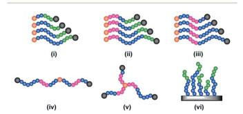
Fig. 5 The range of complex materials synthesised *via* organocatalysed LRP, illustrating a variety of architectures, namely (i) diblock copolymers, (ii) and (iii) triblocks with variation of dispersity of different blocks, (iv) multiblock (v) 3 arm star and (vi) a brush. This figure is adapted from ref. 82 with permission from Wiley.
