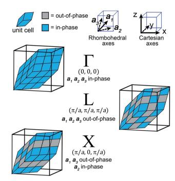
Fig. 3 The translational symmetry, in real space, of the high-symmetry  $\mathbf{k}$  points  $(\Gamma, L \ \delta \ X)$  for the double-perovskite structure.
