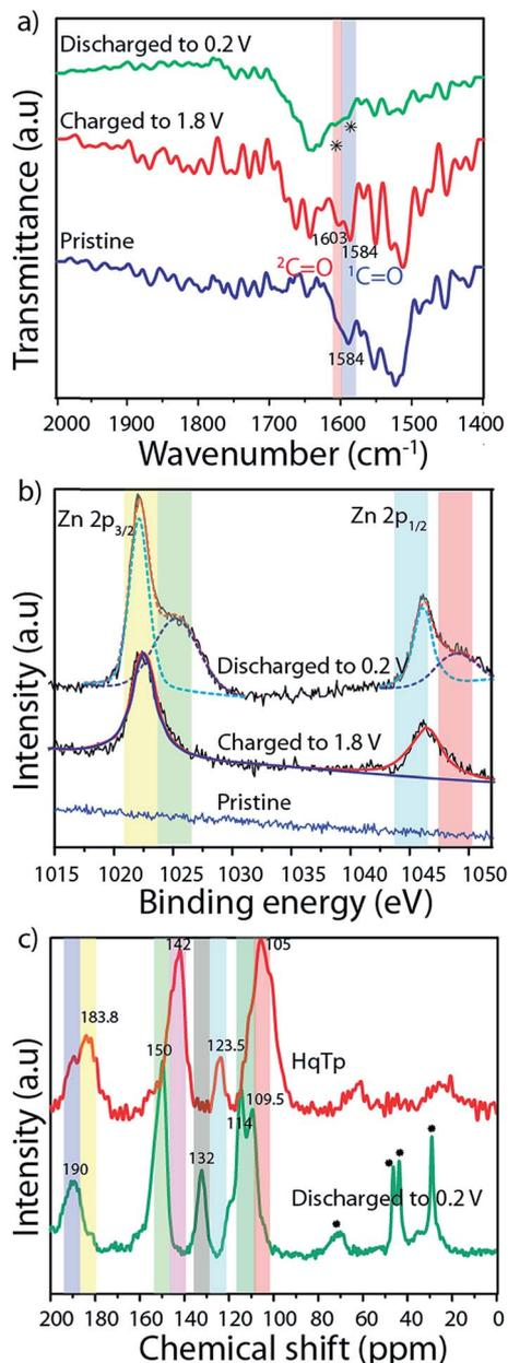
Fig. 2 (a) FT-IR of pristine; charged and discharged cathodes. (b) XPS analysis of pristine; charged and discharged cathodes. (c)  $^{13}\text{C}$  CP-MAS NMR of HqTp and the discharged cathode (all the charging and discharge potential are represented vs.  $\text{Zn}/\text{Zn}^{2+}$  reference).
