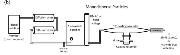
Fig. 3 Schematic of the flow systems for generating (a) polydisperse, coated particles, or (b) monodisperse, coated particles.
