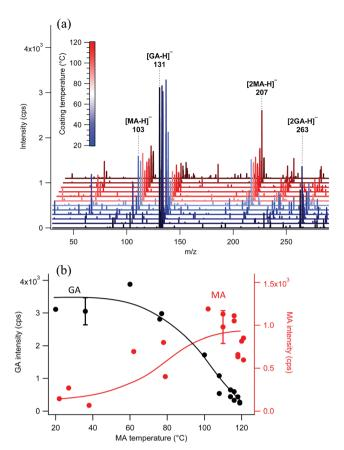
Fig. 5 EASI-MS orthogonal mode analysis of polydisperse glutaric acid (GA) particles coated with malonic acid (MA) at increasing coating reservoir temperatures. (a) EASI-MS spectra collected in orthogonal mode. Spectra were averaged over approximately one minute. (b) Signal intensities of GA (black) and MA (red) as a function of MA coating temperature. Error bars represent 1s standard deviations and the solid lines are guidelines only.
