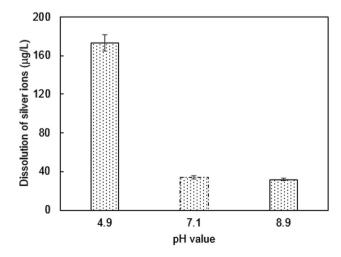
Fig. 7 Dissolution of silver ions in PQAS-AgNPs under different pH values. Reaction conditions:  $[AgNPs] = 10.0 \text{ mg L}^{-1}$ , reaction time = 60 min. T = 25 °C.
