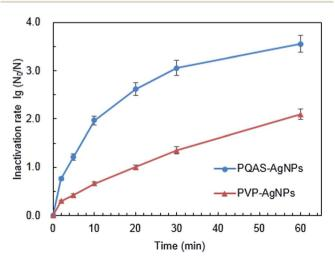
Fig. 2 Inactivation efficiency of *B. subtilis* by PQAS–AgNPs and PVP–AgNPs. Reaction conditions: [AgNPs] = 10.0 mg L $^{-1}$ , pH = 7.1, T = 25 °C, initial concentration of bacteria:  $10^6$  CFU mL $^{-1}$ .
