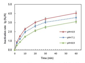
Fig. 6 Inactivation efficiency of B. subtilis with PQAS-AgNPs of different pH values (pH = 4.9, 7.1, 8.9). Reaction conditions: [AgNPs] = 10.0 mg L<sup>-1</sup>, reaction time = 60 min, T = 25 °C, initial concentration of B. subtilis: 10<sup>6</sup> CFU mL<sup>-1</sup>.
