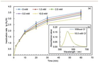
Fig. 8 (a) Effect of Cl<sup>-</sup> on antibacterial efficacy to B. subtilis of PQAS-AgNPs. (b) Ultraviolet absorption spectra of PQAS-AgNPs in electrolyte solution. Reaction conditions:  $[AgNPs] = 10.0 \text{ mg L}^{-1}$ , contact time = 60 min, pH = 7.1, T = 25 °C, initial concentration of B. subtilis:  $10^6$  CFU mL $^{-1}$
