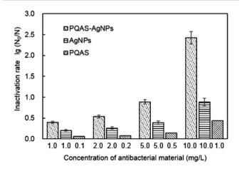
Fig. 5 Inactivation efficiency of *B. subtilis* by different doses of PQAS–AgNPs, AgNPs and PQAS. Reaction conditions: reaction time = 15 min, pH = 7.1, T = 25 °C, initial concentration of bacteria:  $10^6$  CFU mL<sup>-1</sup>.
