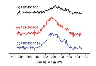
Fig. 4 The high-resolution XPS spectra of the Cl 2p region of chlorinated PETsDQAC0, PETsDQAC8 and PETsDQAC12 nonwovens.
