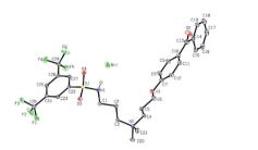
Fig. 3 ORTEP representation of **6a** found in the unit cell and selected bond lengths (Å) and bond angles (°): S(1)-O(3) 1.431(2), S(1)-O(4) 1.433(2), N(1)-C(1) 1.469(4), N(2)-C(3) 1.514(3), N(2)-C(4) 1.514(3), N(2)-C(20) 1.499(4), N(2)-C(21) 1.504(4), O(1)-S(1)-O(2) 119.91(13), O(1)-S(1)-C(22) 107.40(13), O(1)-S(1) 118.8(2), O(3)-S(1)-O(4) 112.5 (2).
