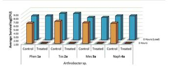
Fig. 8 Survivability of Arthrobacter sp. when inoculated onto plastic coupons treated with compounds 1a-4a, compared against untreated controls. The measurement at 0 h (> $10^7$  CFU for Arthrobacter sp.) indicated the initial number of bacterial cells inoculated onto sample material and was determined concurrently to inoculation, while the measurement at 3 h represents a standardized amount of time to allow the inoculum to dry onto a sample surface (n = 3).
