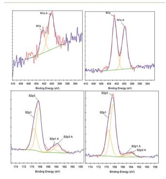
Fig. 5 XPS data corresponding to the nitrogen content (top) and sulfur content (bottom) for control (left) and 3a treated (right) CPVC samples.
