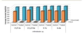
Fig. 10 Survivability of *Arthrobacter* sp. when inoculated onto plastic coupons treated with compounds 5a-8a, compared against untreated controls (n=3).
