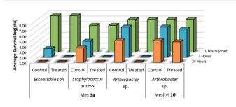
Fig. 13 Survivability of various microorganisms when inoculated onto plastic samples treated with compound 3a and 10, compared against untreated plastic controls. The measurement at 0 h (> $10^7$  CFU for *Arthrobacter* sp. and *Escherichia. coli*, > $10^5$  CFU for *Staphylococcus. aureus*) indicated the initial number of bacterial cells inoculated onto sample material and was determined concurrently to inoculation (n = 3).
