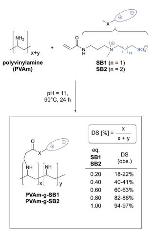
Scheme 1 Reaction of PVAm with sulfobetaine acrylates SB1 and SB2. The range of DS (degree of substitution) of the resulting graft polymers that is shown on the right represents the results of multiple experiments.
