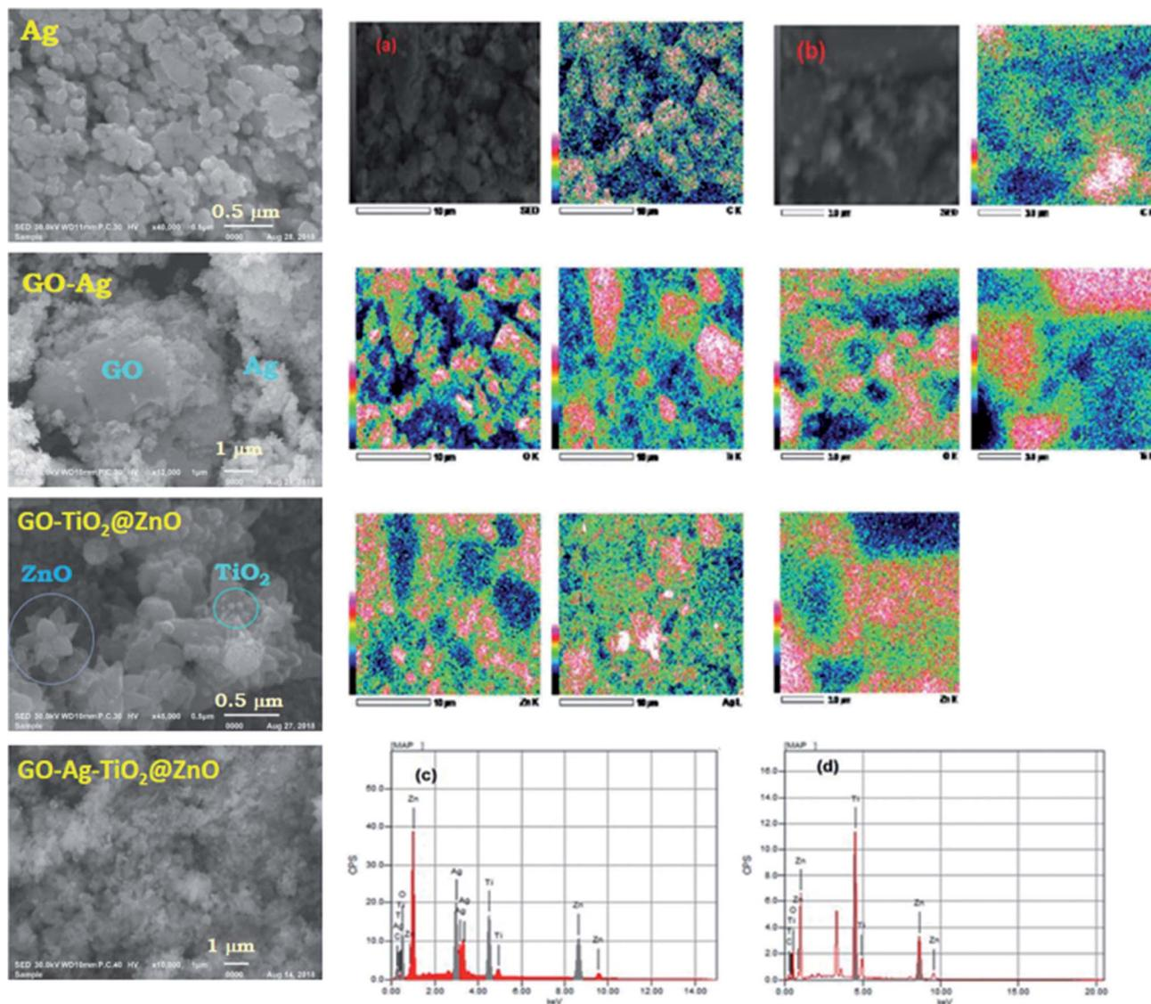
Fig. 2 (Left) SEM images of Ag, GO-Ag, GO-TiO<sub>2</sub>@ZnO, and GO-Ag-TiO<sub>2</sub>@ZnO. (Right) SEM mapping of (a) GO-Ag-TiO<sub>2</sub>@ZnO and (b) GO-TiO<sub>2</sub>@ZnO. (Bottom right) EDX of mapping image of (c) GO-Ag-TiO<sub>2</sub>@ZnO and (d) GO-TiO<sub>2</sub>@ZnO.
