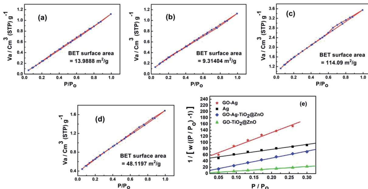
Fig. 5 N<sub>2</sub> adsorption/desorption isotherm curve of (a) Ag, (b) GO-Ag, (c) GO-TiO<sub>2</sub>@ZnO, and (d) GO-Ag-TiO<sub>2</sub>@ZnO nanocomposites. (e) Langmuir fits from the N<sub>2</sub> adsorption data for Ag, GO-Ag, GO-TiO<sub>2</sub>@ZnO, and GO-Ag-TiO<sub>2</sub>@ZnO nanocomposites.
