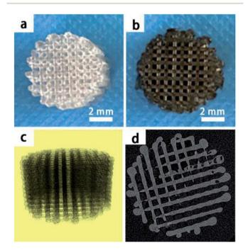
Fig. 2 The macroscopic view of PLGA and pDA-PLGA 3D printed scaffolds (a and b), micro-CT micrographs of PLGA 3D printed scaffolds (c and d).
