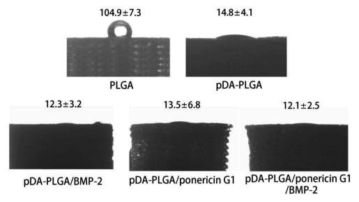
Fig. 5 Water contact angle measurement for the PLGA, pDA-PLGA/BMP-2, pDA-PLGA/ponericin G1 and pDA-PLGA/BMP-2/ponericin G1 scaffolds.
