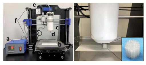
Fig. 1 Schematic diagrams of: (a) temperature controller, (b) receiving plate, (c) heating tube, (d) print nozzle, (e) nitrogen, (f) 3D printer and the printing process of PLGA 3D scaffold.
