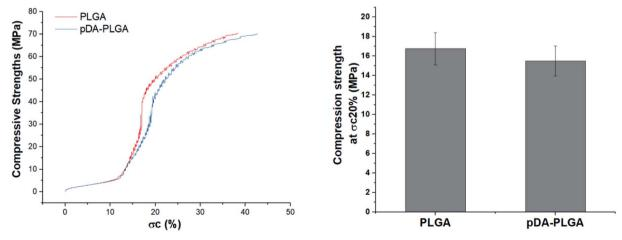
Fig. 4 Compressive strength of the PLGA and pDA-PLGA 3D scaffolds were obtained under a cross-head speed of 2 mm min<sup>-1</sup>. n = 3.
